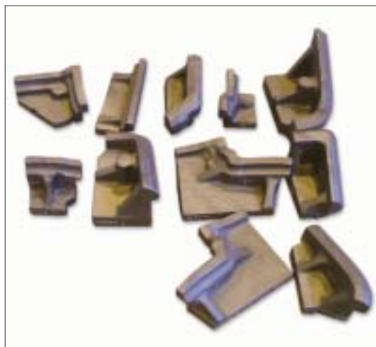
Automotive tool parts cast via polystyrene model and Uddeholm Carmo Granshots.
