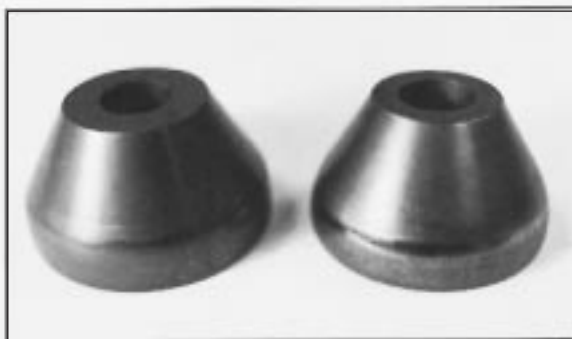
PVD coated tools in VANADIS 23 for cold forming of tubes.
