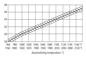
Hardness for different austenitizing temperatures after tempering 3 times for one hour at  $560^{\circ}C$  ( $\pm 1$  HRC)
