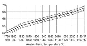
Hardness for different austenitizing temperatures after tempering 3 times for one hour at 1040°F (560°C) ( $\pm 1$  HRC).
